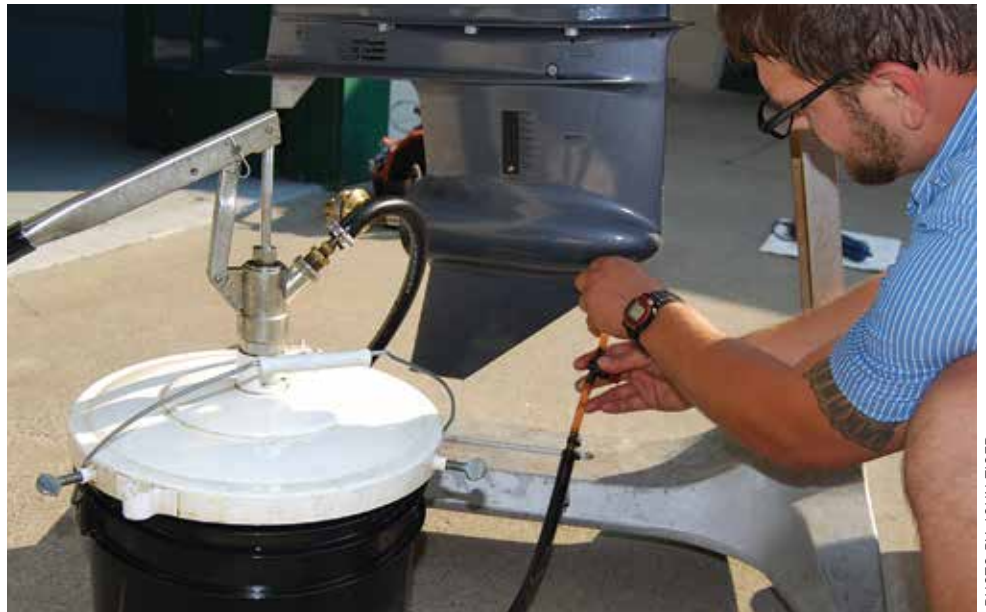
Changing the lower unit oil will help protect your boat from worn out lube over the winter.
