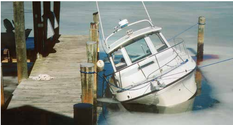
Boats stored in water over winter are vulnerable to sinking damage if a hose or thru-hull fails.
