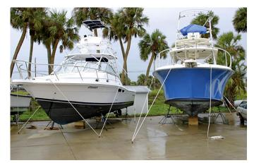
Left: Boats that are hauled out are far less likely to be damaged during a storm than those left in the water. Using straps is effective at keeping boats from toppling over or floating away. Below: Lines should be extra long to allow for surge. Double up lines where possible.
