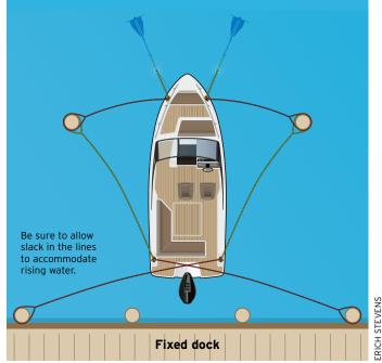
If you don't have a slip, tie extra-long lines to pilings or cleats to allow for the surge, which could be 10 feet or more. Use anchors or long spring lines to keep the boat from striking the dock.
