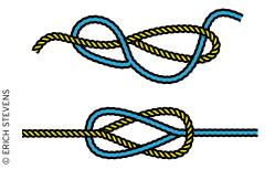
By joining a polyester line from the cleat through the chock to nylon line from the piling or mooring, you can get the best of both types of line – the chafe resistance of polyester and the stretch of nylon.
