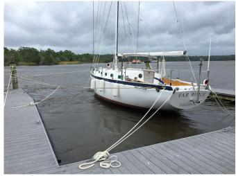
strand lines; there's nothing hidden under an outer cover as with double-braided. As an added precaution, we doubled all docklines for added strength and to provide redundancy should a line break
