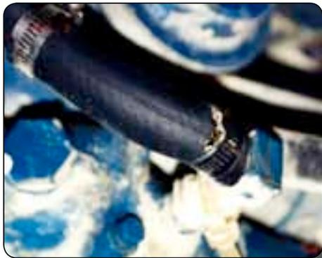
**A combination of a too-tight hose clamp and age caused this hose to leak gasoline. A surveyor doing a pre-purchase survey averted a catastrophe (Claim #0001161).**
