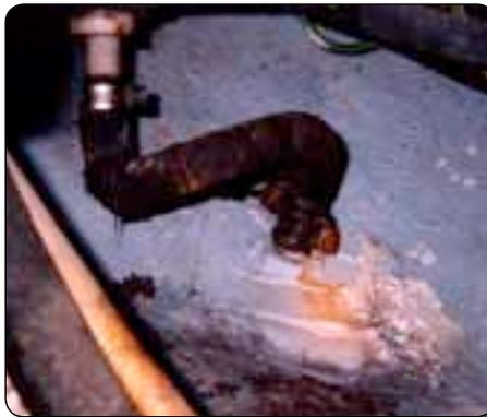
Hoses that are hard to reach don't always get inspected. This hose is completely shot, yet its job is to carry explosive propane out of the propane locker. Note that it's also connected to a threaded fitting, rather than a proper barb (Claim #0300044).
