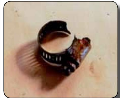
Good quality hose clamps last much longer than cheap ones. Look for clamps that are 100% stainless steel (including the screw). The best ones are non-perforated rather than slotted. Rust tends to form on the lowest part of the clamp—it's a good idea to rotate them periodically to check for corrosion.
