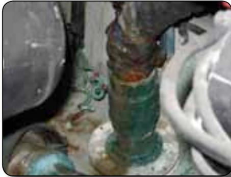
The only thing between this boat's hull and the water is this hose, which is so old the reinforcement wires have rusted through. Note also the broken clamp; this boat could sink at any time.
