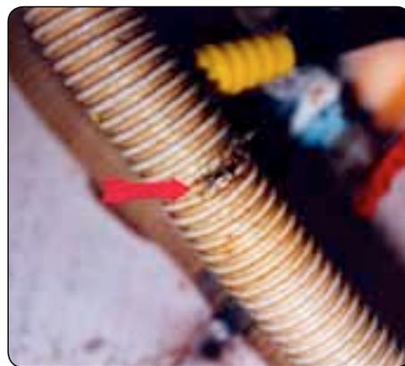
**This bilge pump hose is ridged, which adds significant friction and decreases the bilge pumps' performance. Ridged hose is also not nearly as strong as smooth-walled hose and is much more easily damaged. This hose chafed against a vibrating engine and bilge water simply dumped back into the bilge (Claim #0110782).**
