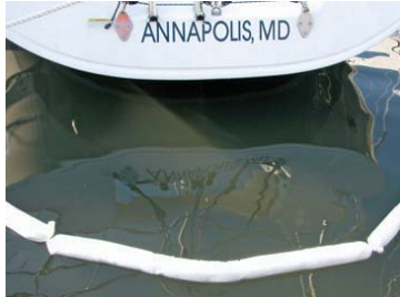
Spill Booms Typically sausage-shaped absorbents, in 4' lengths or longer, and can be hooked together. Put around a boat, dock or large spill.
