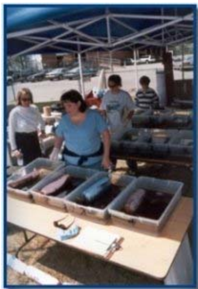
12 Pillows in "bilge water" are timed to soak up oil.
