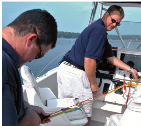
We measured the length of the kill switch lanyards to see how much freedom of movement would be possible with each.
