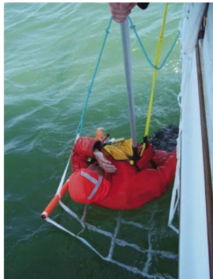
The Markusnet scramble net can also be used to "roll" a victim back on board.
