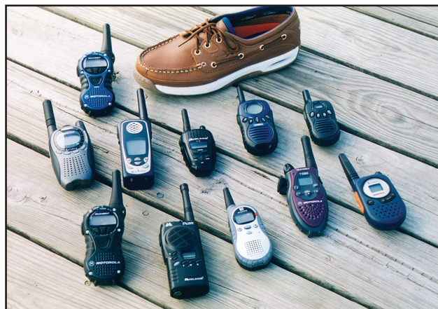
Testing entailed reading scripted sentences over the air at half-mile intervals. Eleven models of FRS and GMRS radios (at right) were tested on land and water.
