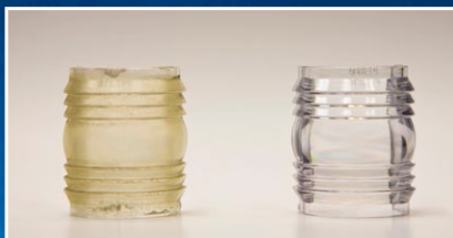
Our 11-year-old lens (on the left) appears cloudy and can be replaced for less than $15.
