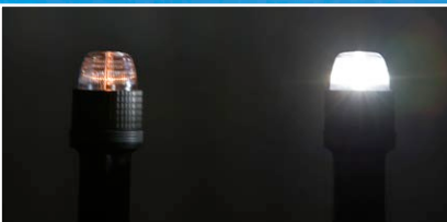
Top: Incandescent and LED versions of the same fixture with brand new batteries. Bottom: The same two fixtures after five hours of continuous use; the incandescent quickly died.
