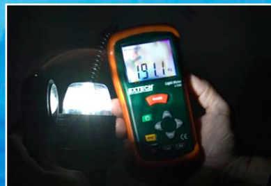
A light meter, used in a darkened room, records brightness in foot candles (Fc).
