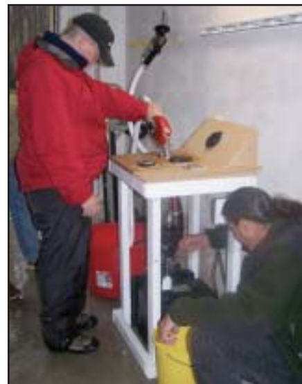
To test the hardware, we built a mock-up of a boat fuel tank system, complete with a tank vent.
