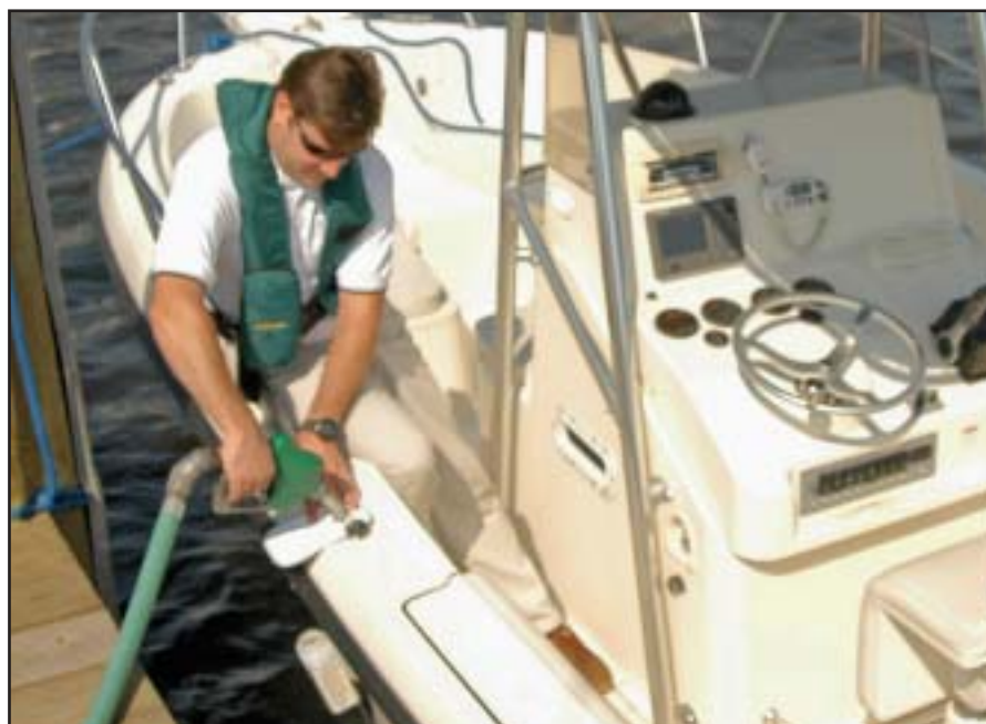
Using products like this nozzle bib and No Spill catchment device can also help prevent accidental spills.
