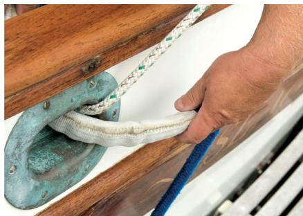
**Top: Lines led perpendicular from a cleat can wrench the cleat out of the deck. Two-hole cleats are more vulnerable than four-hole cleats. Above: Chafe protection is essential on all lines where they rub against chocks, pilings, or the dock itself.**
